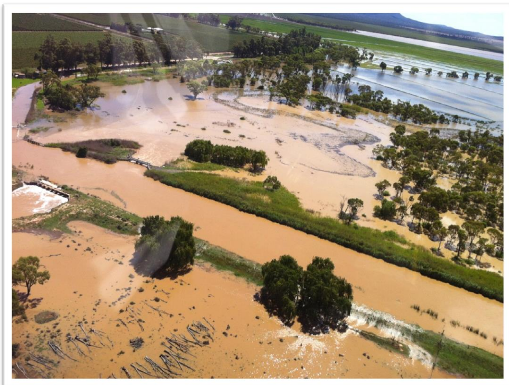
Figure 8-27 Main Canal Overtopping at the EMR during the March 2012 Flood Event
