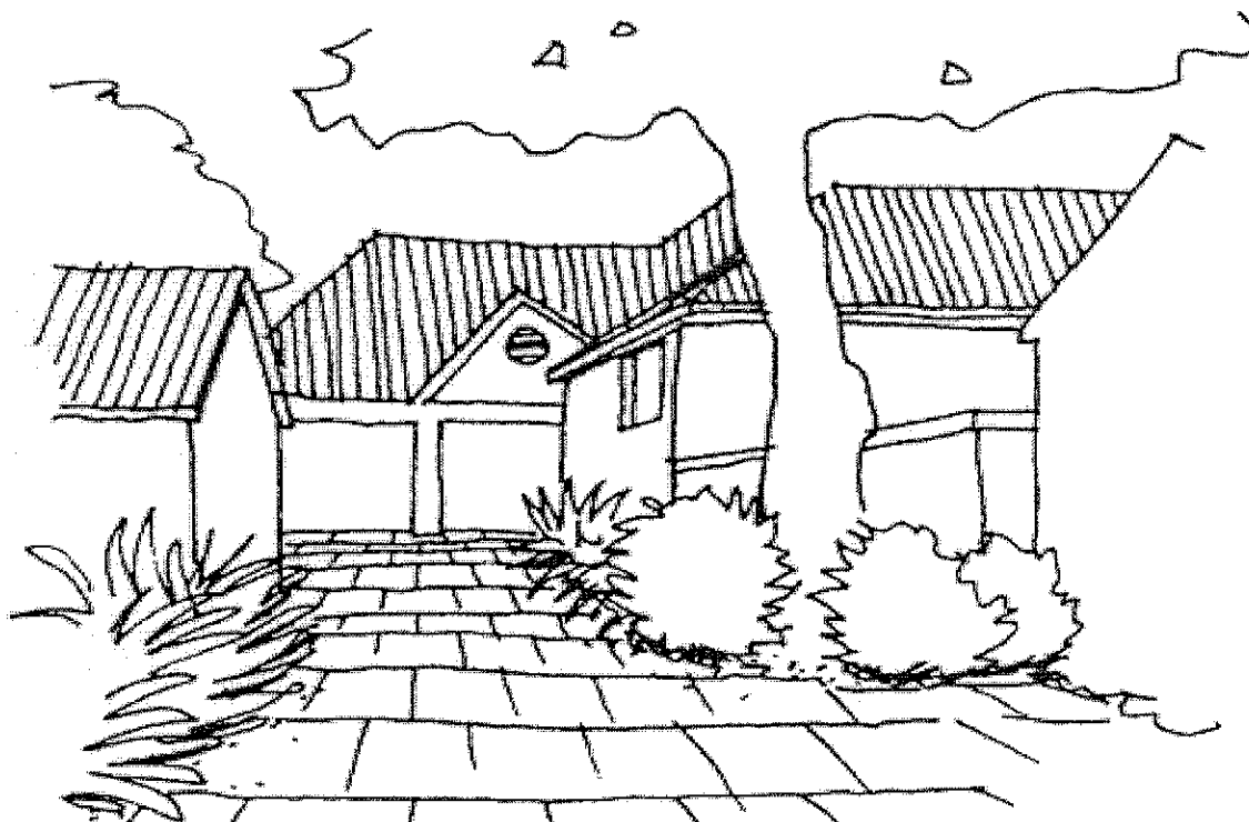
FIGURE 40. Pervious landscaping adjoining paved areas, reduce stormwater run-off. (Source: Amcord.)
