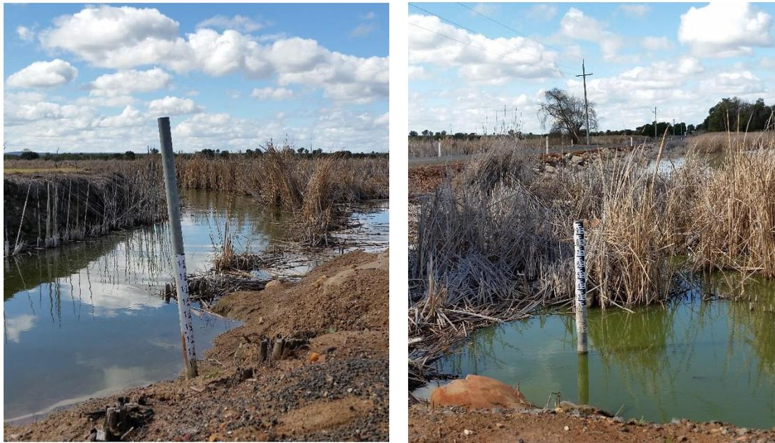
**Figure A1** Water level gauges reading: 1.0m for the Northern Lake (left) and 0.8m for Southern Lake (right) at time of survey
